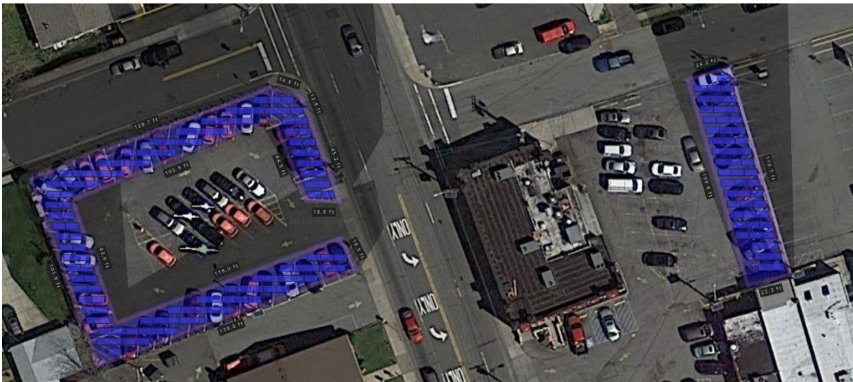
Figure 2. Reo Diner Helioscope Solar PV Mock-up
